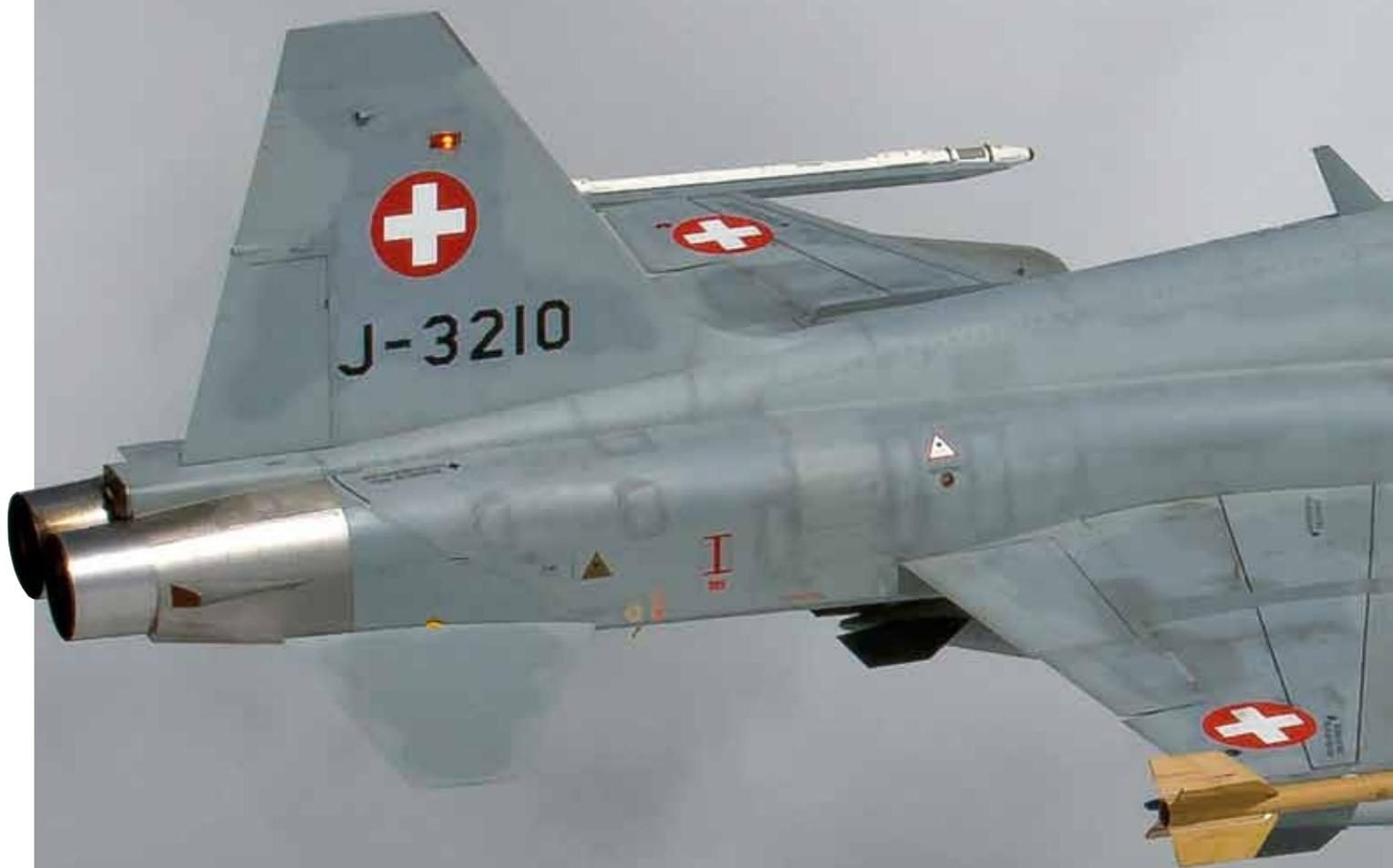
*Anonymous two-seat F-5F J-3210 carrying an AIM-9P5 Sidewinder training round on the starboard wing-tip weapons rail, seen high over Switzerland.*
