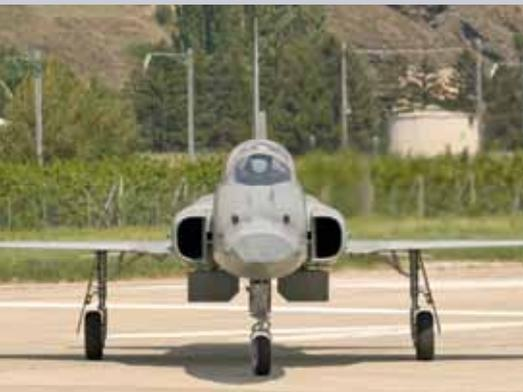
**Above: The F-5E is equipped with a double 20mm M39 cannon capable of firing 1,500 rounds per minute. The gun is primarily intended for air combat but ground attack is practised at the Ebenfluh/Axalp shooting range. The F-5F only carries one cannon.**
