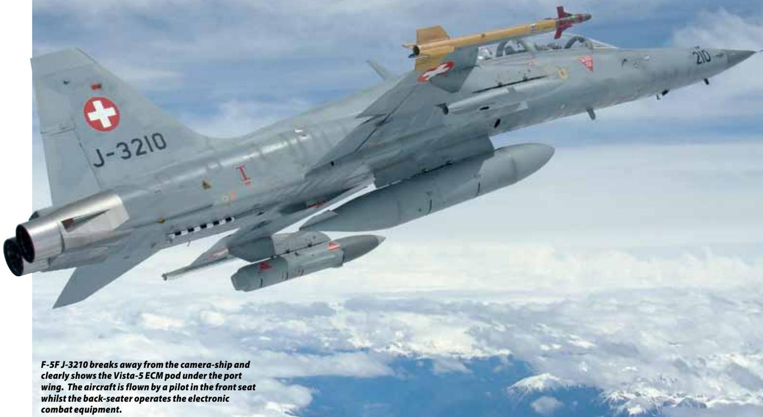
**F-5F J-3210 breaks away from the camera-ship and clearly shows the Vista-5 ECM pod under the port wing. The aircraft is flown by a pilot in the front seat whilst the back-seater operates the electronic combat equipment.**
